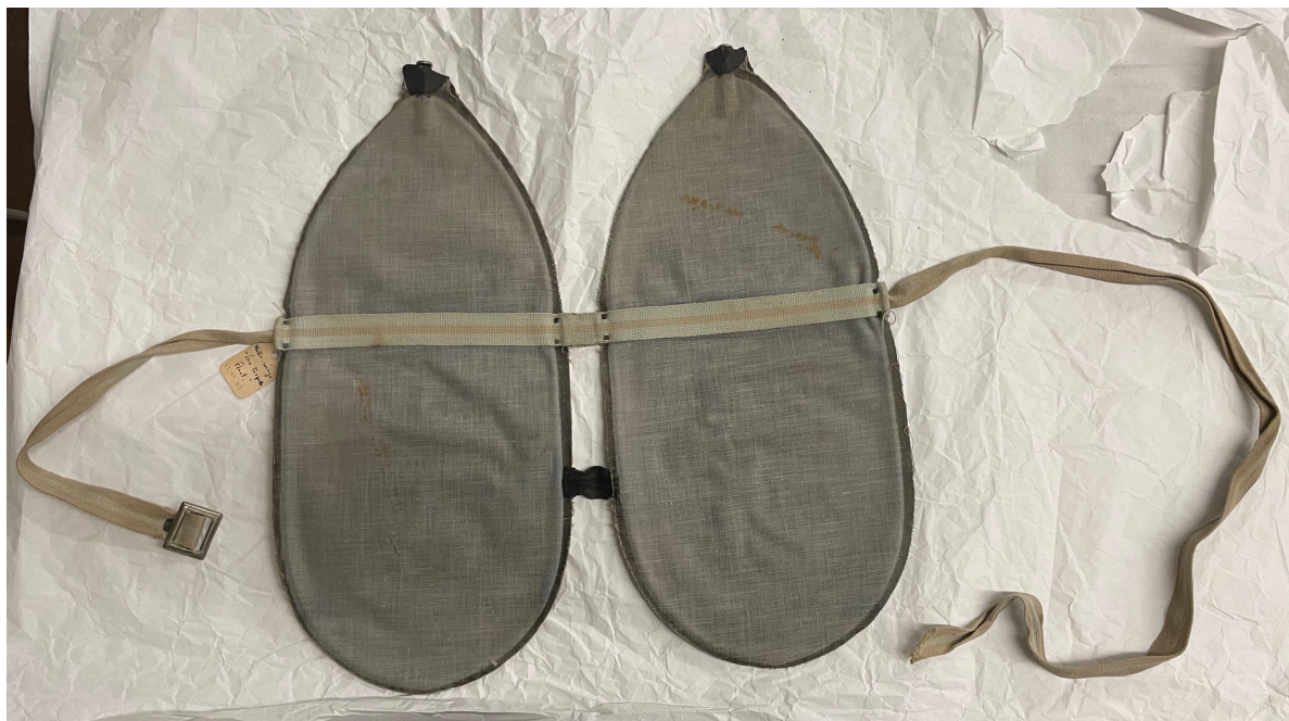
Figure 2: Inner side/Bottom of The Torpedo Float
